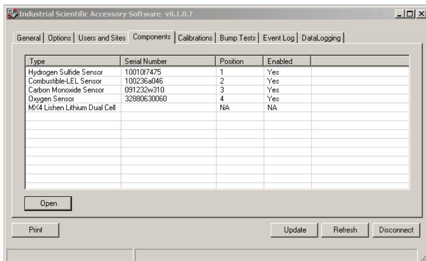
**Figure 8.** Components tab.
