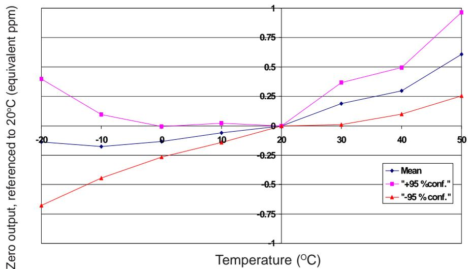
Figure 3 shows the variation in zero output caused by changes in temperature, expressed as ppm gas equivalent, referenced to zero at  $20^\circ\text{C}$ .
