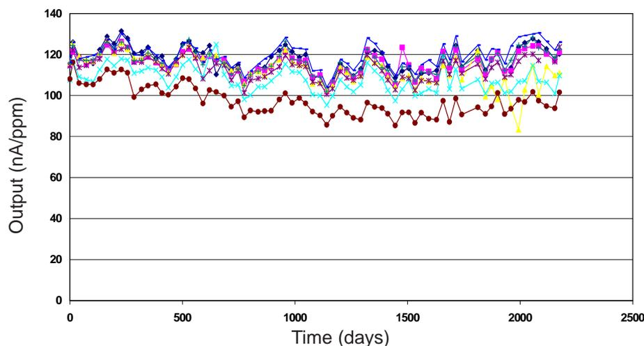
Figure 4 shows the long term stability of the H2S-D4 sensitivity in ambient air.
