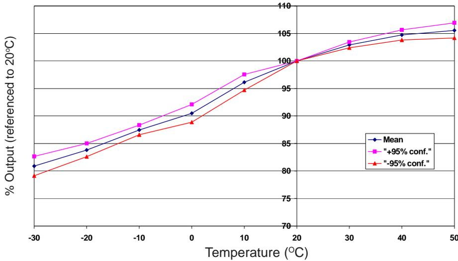
Figure 2 shows the mean and  $\pm 95\%$  confidence intervals for the variation in sensitivity caused by changes in temperature.
