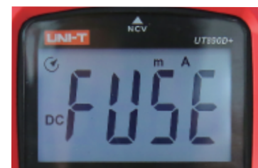
Fuse blowing alarm (mA only)
